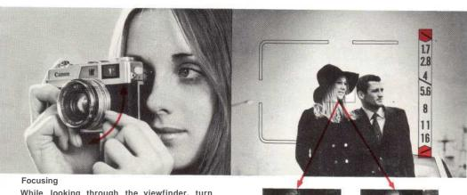
While looking through the viewfinder, turn the focusing lever. The subject is in focus when the double image merges into one precise image in the center of the viewfinder.
